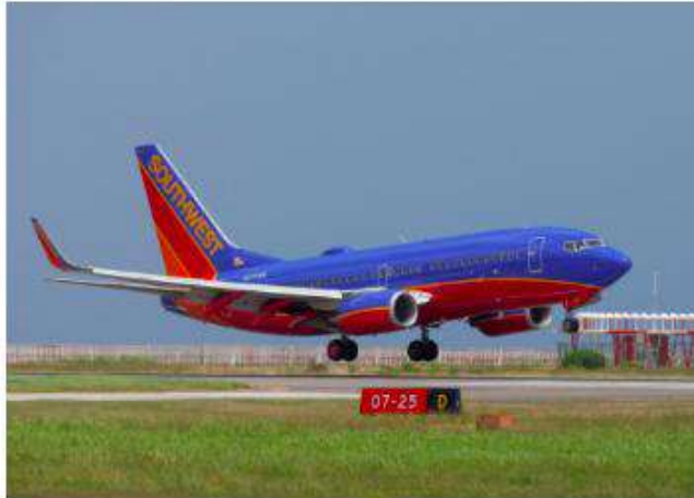
Blended Winglets (first installations began in 2007); fuel savings of about 3.5 percent per aircraft.
